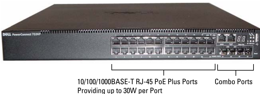
Figure 1-2. PowerConnect 7024P with 24 10/100/1000BASE-T PoE Plus Ports
